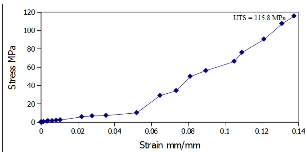
**Fig. 7.** Stress–Strain Curve for Al6061-12% Graphite.
