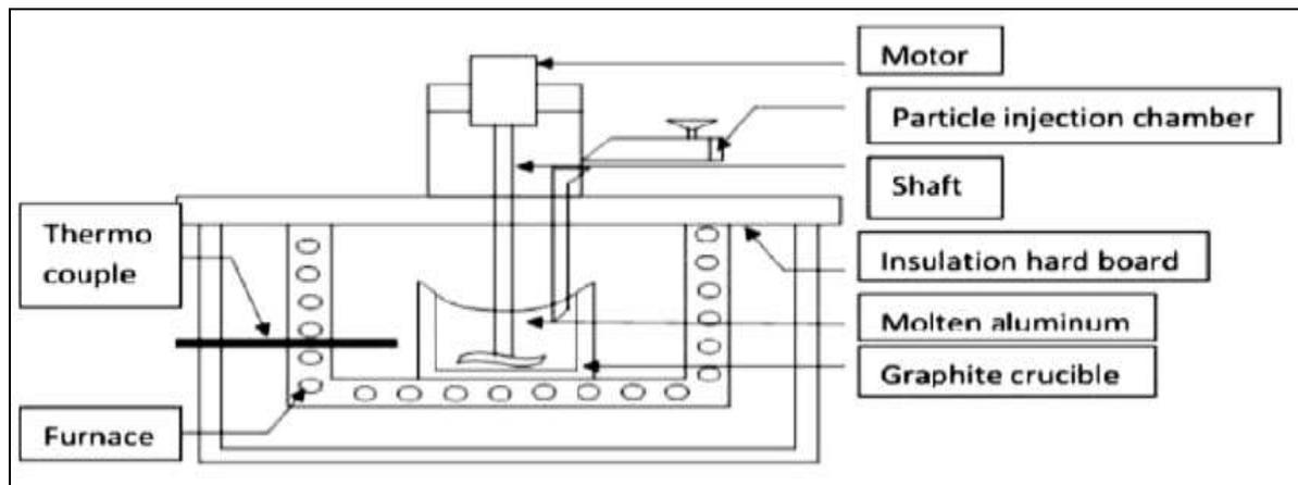
**Fig. 1.** Schematic View of Stirring Mechanism Used in the Fabrication of MMC.<sup>[4]</sup> [Source: [www.ijert.org](http://www.ijert.org)].
