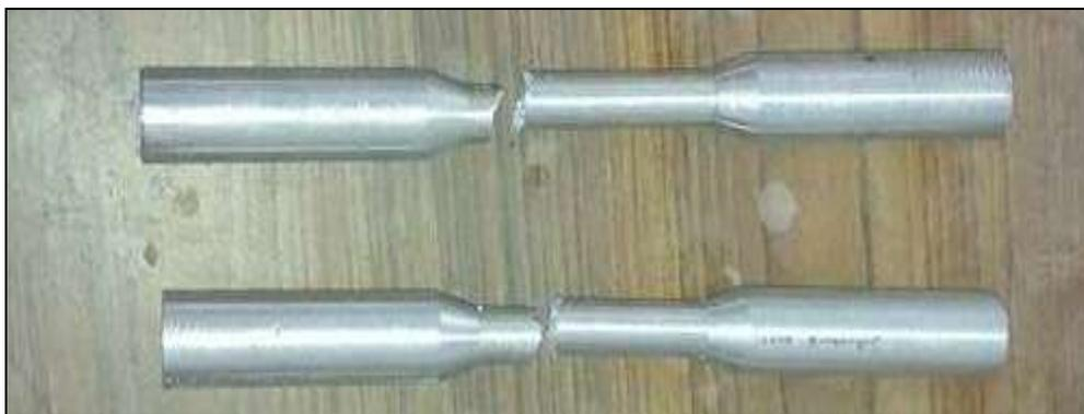
*Fig. 3. Tensile Test Specimen After Testing.*
