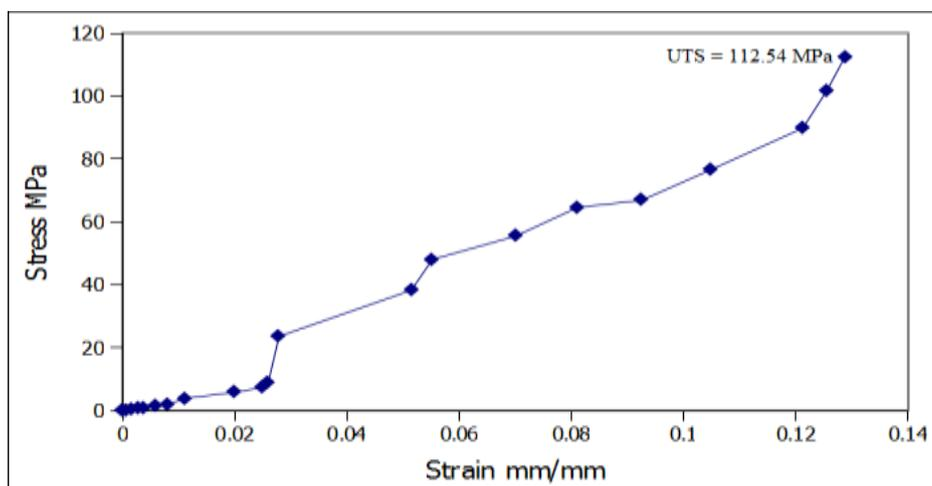
*Fig. 4. Stress-Strain Curve for Al6061-3% Graphite.*
