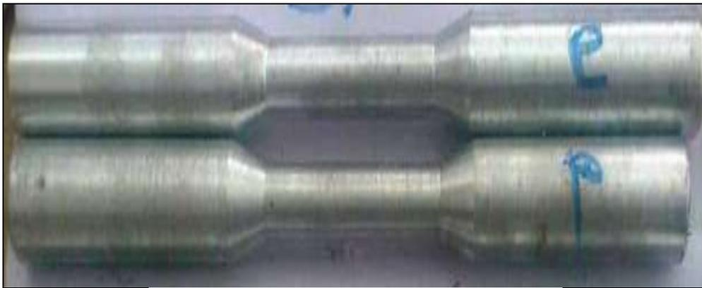
*Fig. 2. Tensile Test Specimen Before Testing.*
