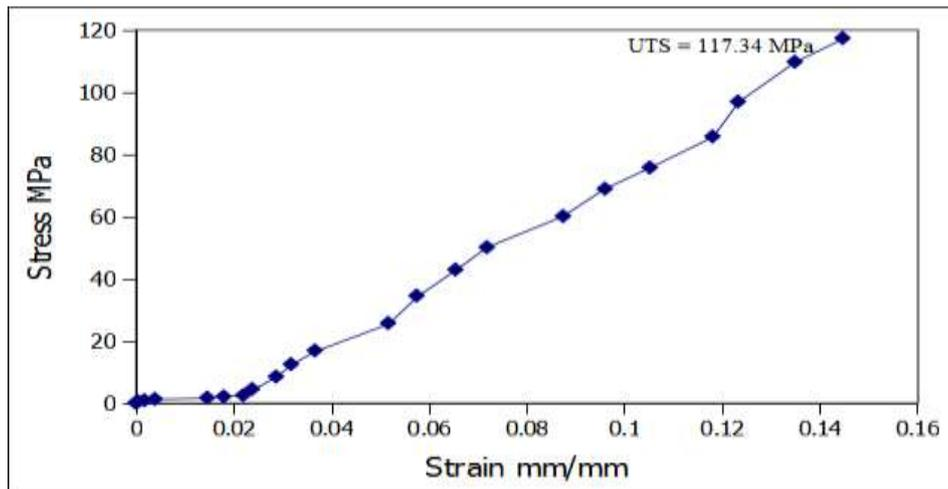
**Fig. 6.** Stress–Strain Curve for Al6061-9% Graphite.
