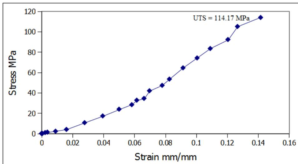
*Fig. 5. Stress–Strain Curve for Al6061-6% Graphite.*
