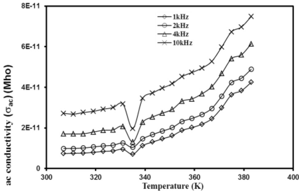
Fig 10: AC Conductivity ( $\sigma_{ac}$ ) for PP with 20% of Cenosphere.
