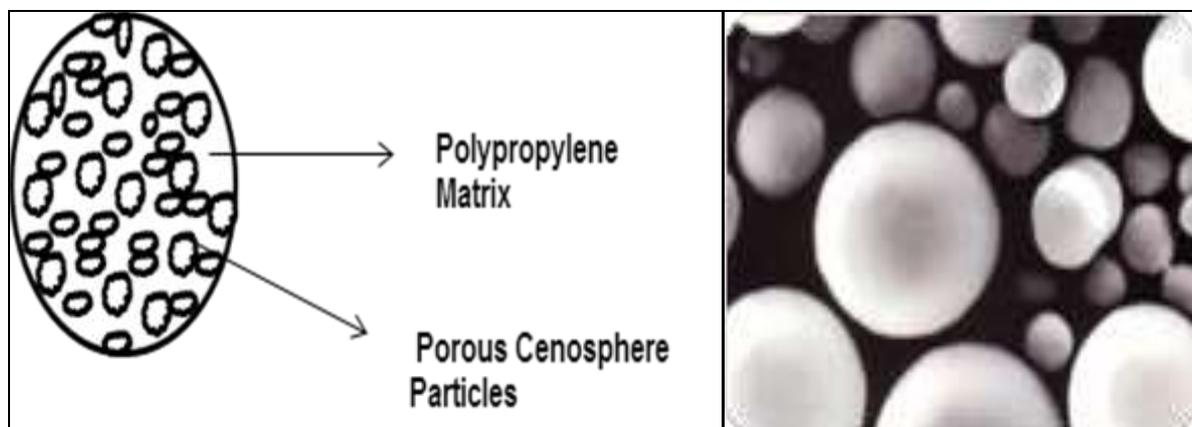
*Fig 1: Schematic of Composites.*
