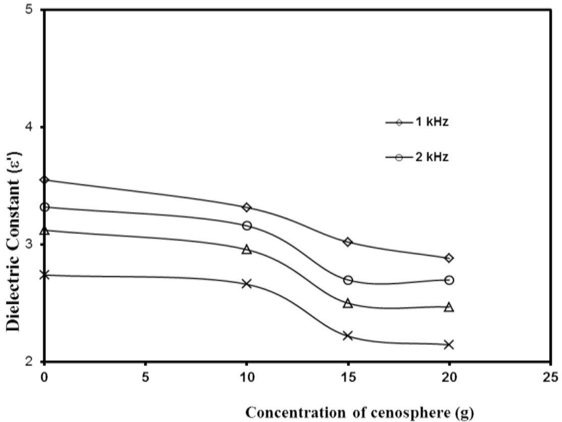
Fig 6: Variation of Dielectric Constant for Different Volume Fractions of Cenosphere.
