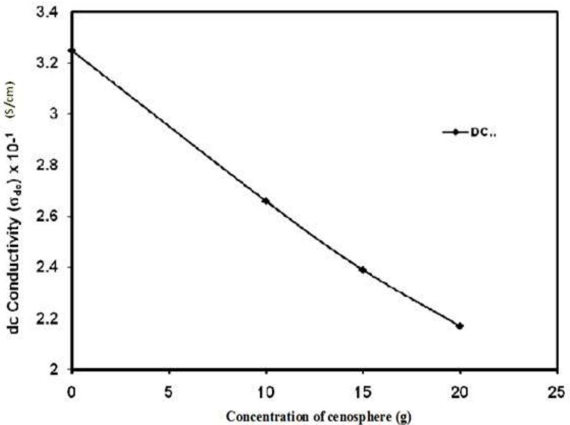
Fig 7: DC Conductivity for Different Weight Percentage of Cenosphere.
