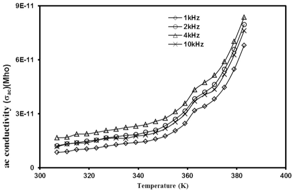
Fig 9: AC Conductivity ( $\sigma_{ac}$ ) for Pure PP.
