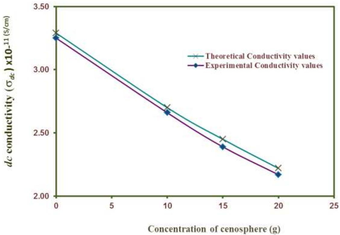
Fig 8: Experimental & Theoretical DC Conductivity for Different Weight Percentage of Cenosphere.
