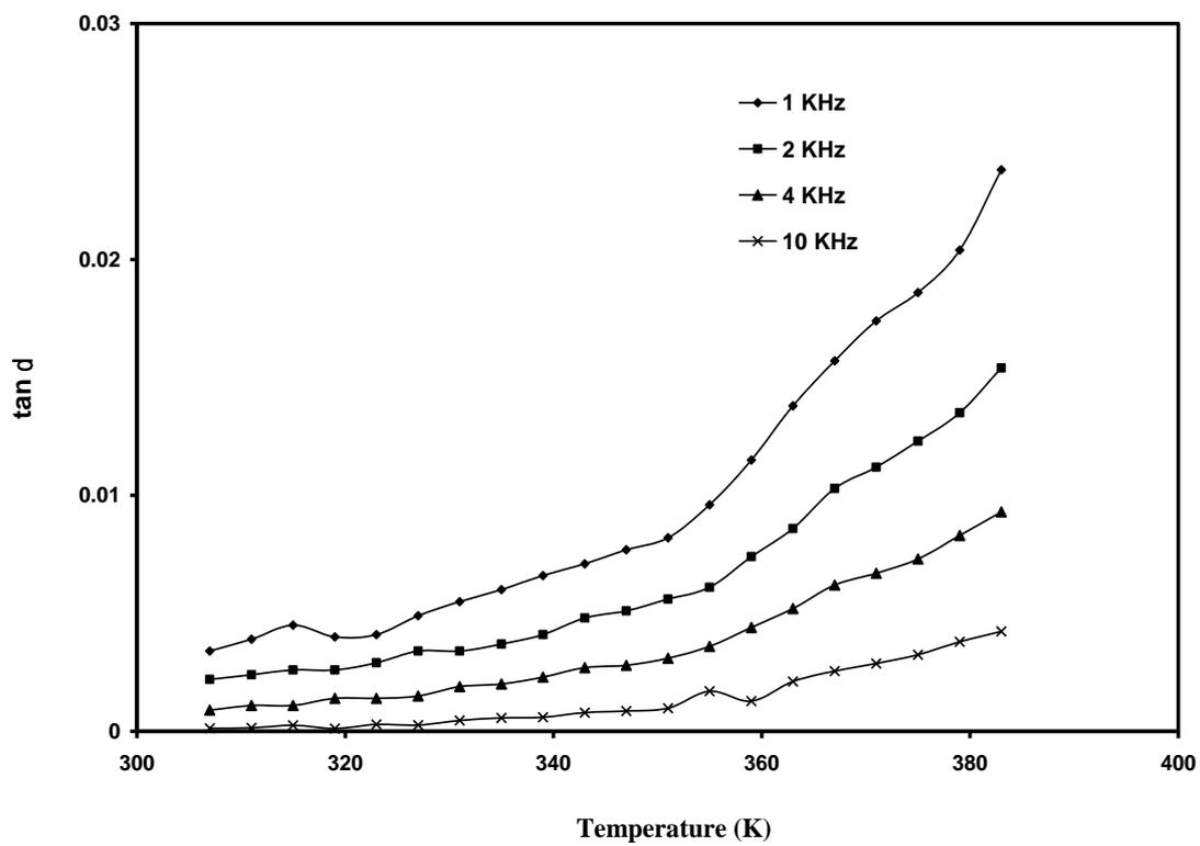
Fig 4: (a) Dielectric Constant & (b) Dissipation Factor for 85% PP with 15% Cenosphere.
