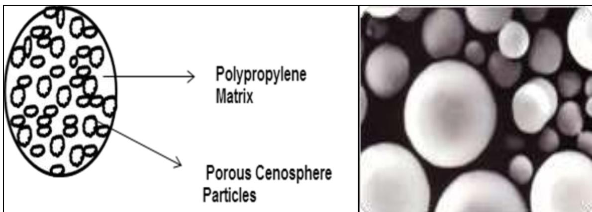
*Fig 1: Schematic of Composites.*
