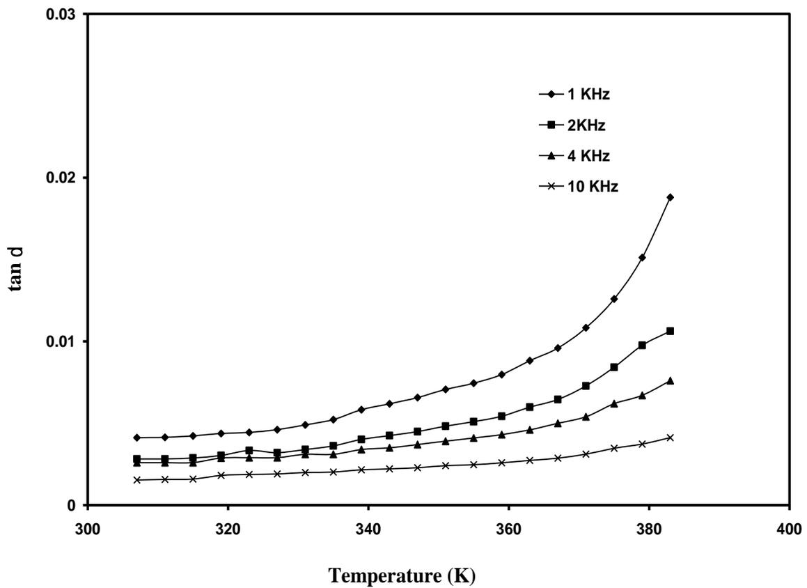
Fig 3: (a) Dielectric Constant & (b) Dissipation Factor for 90% PP with 10% Cenosphere.
