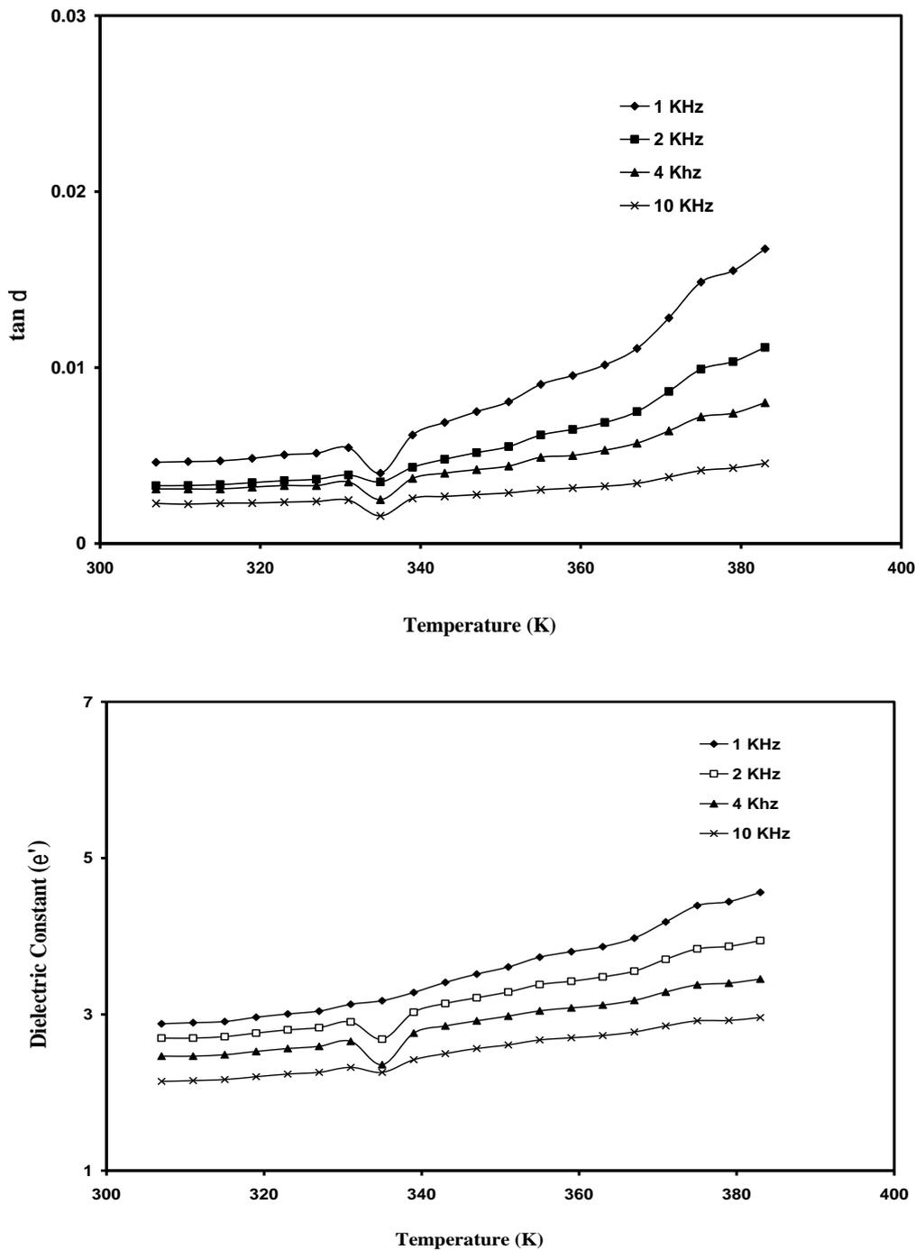
**Fig 5:** (a) Dielectric Constant & (b) Dissipation Factor for 80% PP with 20% Cenosphere.
