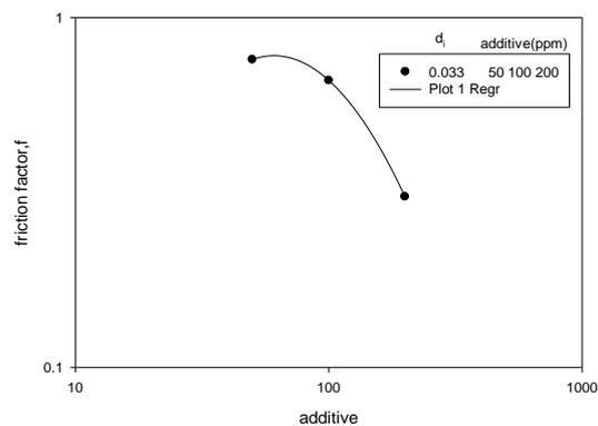
Fig 8 friction factor vs PAA concentration
