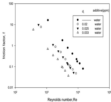
Fig 4  $f$  vs  $Re$  for water-Effect of annular pipe diameter
