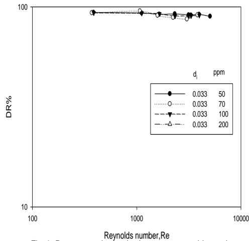
Fig. 3 Percentage drag reduction versus Reynolds number- Effect of polyacrylamide concentration.
