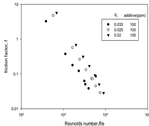
Fig 5  $f$  vs  $Re$  with PAA additive to water- Effect of annular pipe diameter
