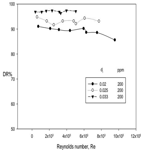
Fig. 2 Variation of drag reduction with Reynolds number- Effect of annular pipe diameter.
