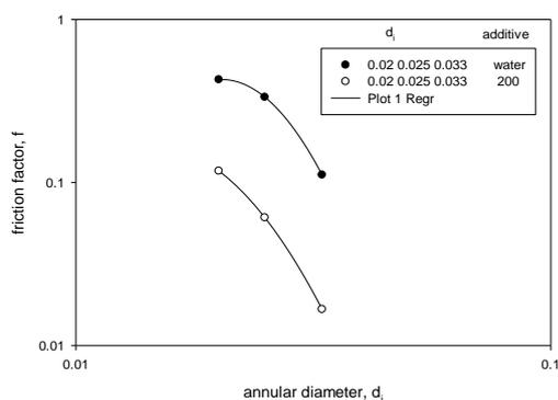
Fig 7 friction factor vs annular pipe diameter
